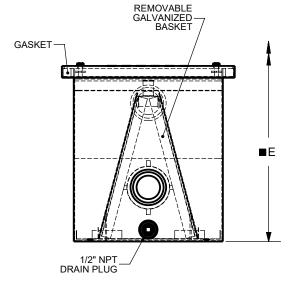
■ Minimum height required for removal of solids basket. If "-EXT" option is supplied, add extension height to this dimension.
